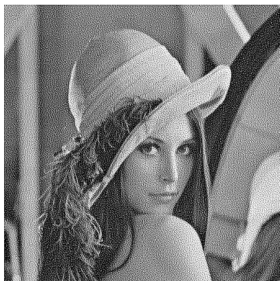
(b) Our proposed watermarked Lena image with 10080 bits embedded, K_w=2.0771
